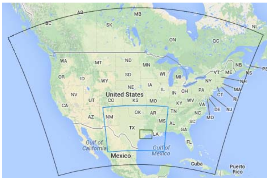
Figure 2. CAMx modeling domain with outer 36 km grid and nest 12 km (blue) and 4 km (green) grids.
